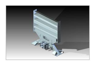
The QuadGuard family has evolved again! Using the existing framework of the QuadGuard, the QuadGuard II provides TL-2 and TL-3 protection using less length. The TL-2 QuadGuard II is 25% shorter than the original QuadGuard measuring less than 3m (10'). The TL-3 model is also nearly a meter, 3 feet, shorter than its predecessor.
