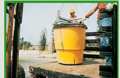
Because of their convenient, one-piece construction, filled Energite III modules can be moved using a special lifting device, if desired.
